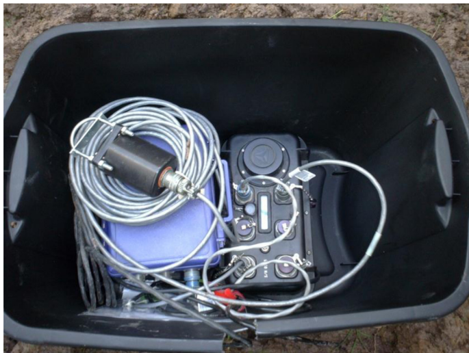
Fig. 15.7. The RefTek RT130 seismometer recorder, with three-component Mark Products model L22, 2.0 Hz geophone. Photograph courtesy of B. Voight.
