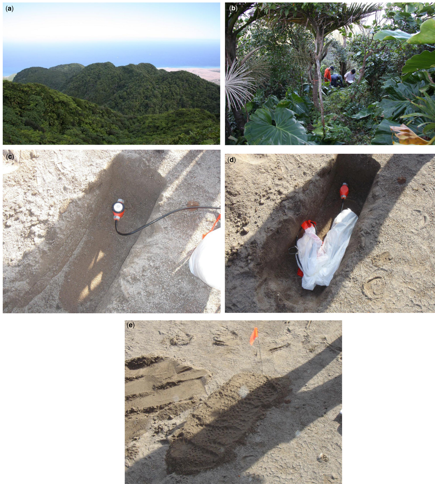
Fig. 15.13. Installation of Texan seismometer stations. Texans were installed in December 2007 just before the airgun shooting. (a) Hikers carried Texans across rugged terrain of the Centre Hills, mountainous rainforest with steep ridges and valleys. Trails on precipitous wet slopes could be almost invisible because of dense vegetation, and were cleared with machetes shortly before the experiment. Photograph courtesy of B. Voight. (b) Installation on the north–south Texan array line on top of Katy Hill (near the words ‘Centre Hills’ in Fig. 15.9), in elfin cloud-forest vegetation with thick undergrowth. Photograph courtesy of A. Belousov. (c)–(e) Sequence showing the Texan installation. Pit with a seismometer and bubble level; seismometer plus datalogger in a protective bag prior to burial; view after the burial with a location flag. Photograph courtesy of G. Mattioli.
