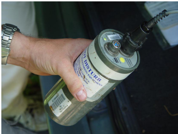
Fig. 15.8. The RefTek RT125A seismometer ('Texan'), with cable to a single vertical component Mark Products L40 (or L28) 4.5 Hz sensor. Photograph courtesy of B. Voight.
