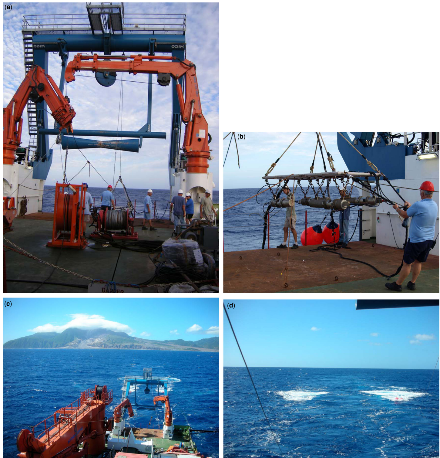
Fig. 15.18. Airgun operations during JC19 on the RRS James Cook . (a) Hoist operations on stern rear deck. Photograph courtesy of J. Hammond. (b) Airgun cluster being prepared for deployment off the stern. Photograph courtesy of J. Hammond. (c) Shooting on a radial track offshore eastern Montserrat. Airgun explosion bubbles are visible behind the hoist. The Tar River Valley leading up to the Soufrière Hills Volcano is in the distance with the volcano summit covered by cloud cap. Photograph courtesy of S. Sparks. (d) Synchronized explosions from the dual airgun clusters, offshore Montserrat. Photograph courtesy of S. Sparks.
