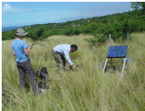
Fig. 15.11. Installation of RefTek seismometer stations. (a) The RefTeks were deployed from October through to December 2007, powered by deep cycle batteries with solar panel recharging. Typical site, at M10 Royal Palm, in partly foliated terrain with buried seismometer and plastic container for the datalogger and battery. Frame with a solar panel in the rear. Photograph courtesy of V. Miller. (b) Site installation at M15 Air Studios. Photograph courtesy of B. Voight.
