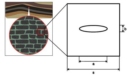
Fig. 1. Dual-porosity fractured medium.
