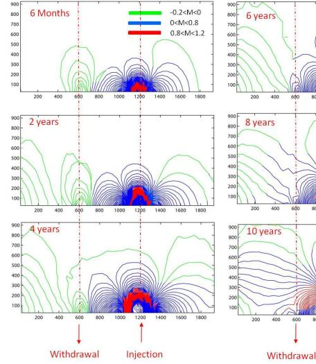
Plots of the potential for triggered seismicity relative to injector
