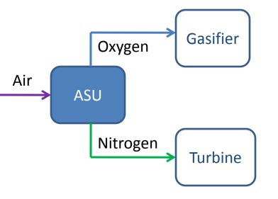
Nitrogen is used as diluent for gas turbines to reduce NOx emissions.
