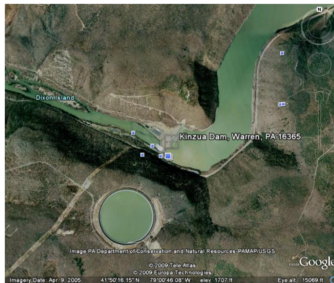
Figure 5 Google Earth™ image for Kinzua Dam and Seneca PHS Station (2080 ft) near Allegheny Reservoir (1330 ft) below
