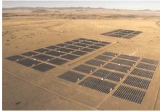
Figure 14: Tucson Electric Power Company's 4.6 MW dc photovoltaic power plant. [41]
