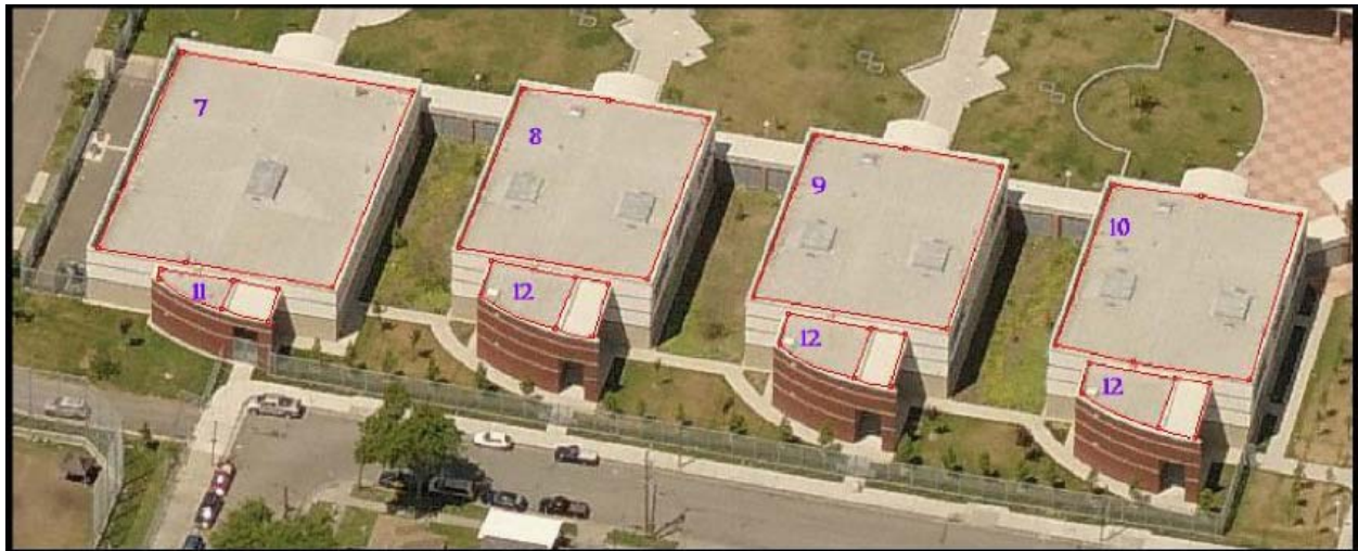
Figure 7.1 Processed Aerial Images for perimeter detection
