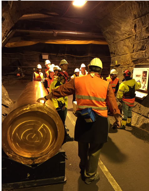
Copper Canister that Houses Spent Fuel Rods
